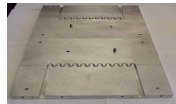
Fig. 1. 2-piece X-band FWG test circuit
